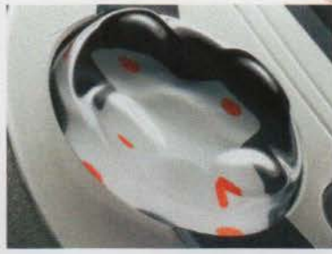
The 'click' function of the original D-pad has been abandoned and set to a separate 'confirm' button, making menu navigation easier and accident-proof.
